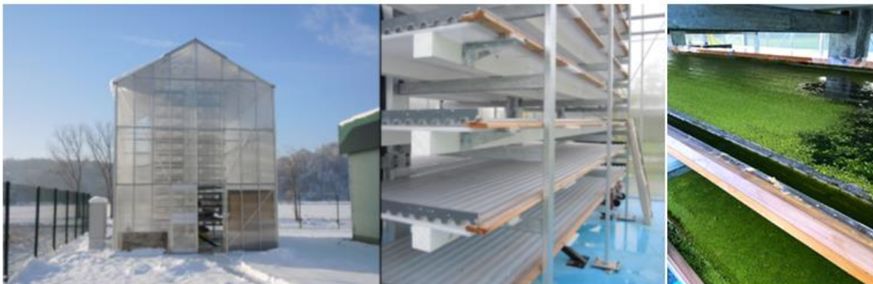
Figure 4: Full scale duckweed pilot plant (left) with detailed picture of the trays (middle) and trays with duckweed during operation (right)
