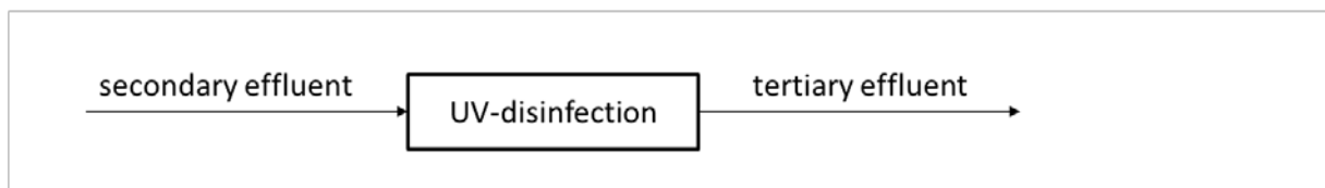
Figure 1 Basic flow sheet for UV disinfection
