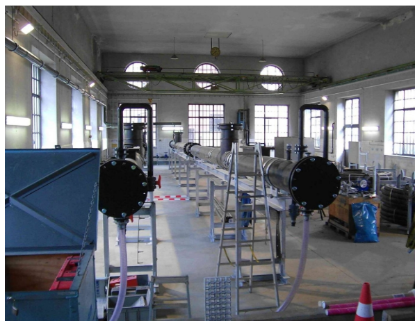
Sewer research plant of Berliner Wasserbetriebe. Site for the test of electronic noses
