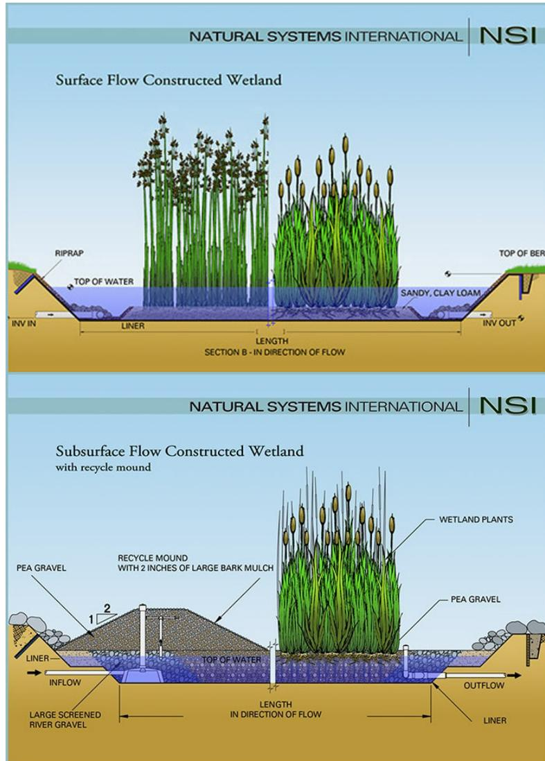
Figure 3 Diagrams comparing the design of surface flow constructed wetlands to subsurface flow constructed wetlands. (www.natsys-inc.com)
