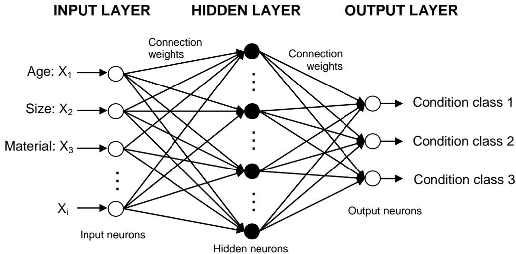
Figure 8: Schematic presentation of the back propagation neural network BPNN (adapted from Tran *et al.* (2007))
