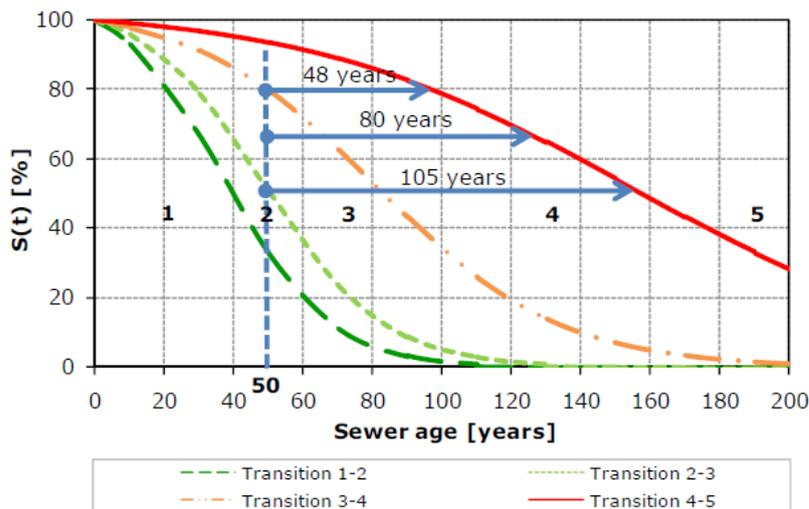
Figure 5: Transition functions for a Norwegian network and prediction of the sewers remaining service life (from Hörold (1998) cited by Ana (2009)).
