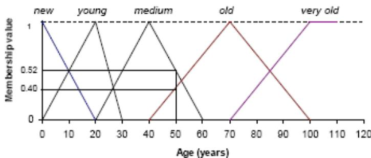
Figure 10: Fuzzy set representation of the condition of a 50 years old pipe (from Kleiner *et al.* (2006) cited by Marlow *et al.* (2009))
