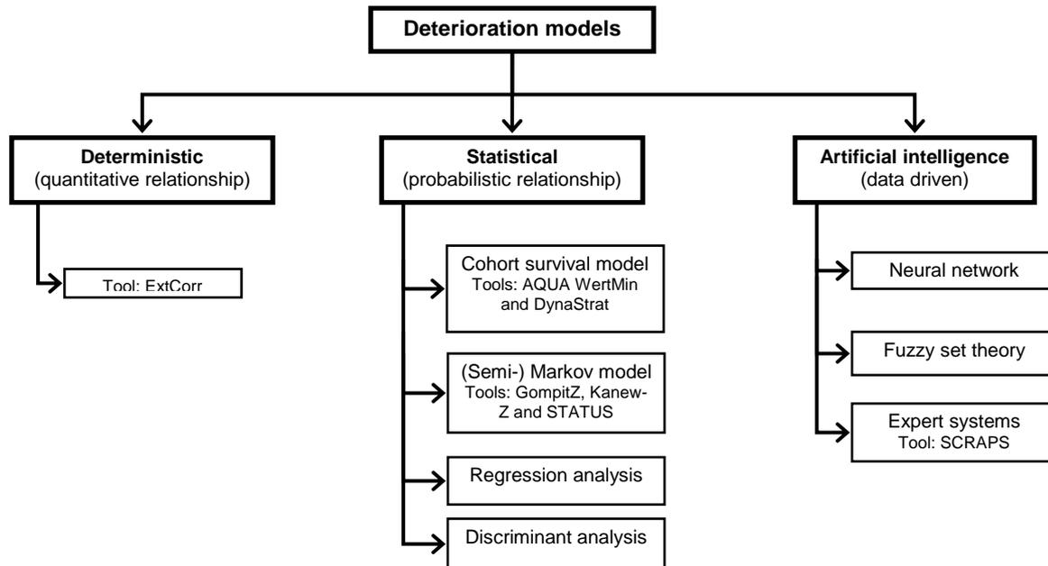
Figure 3: Overview of the different types of sewer deterioration models.
