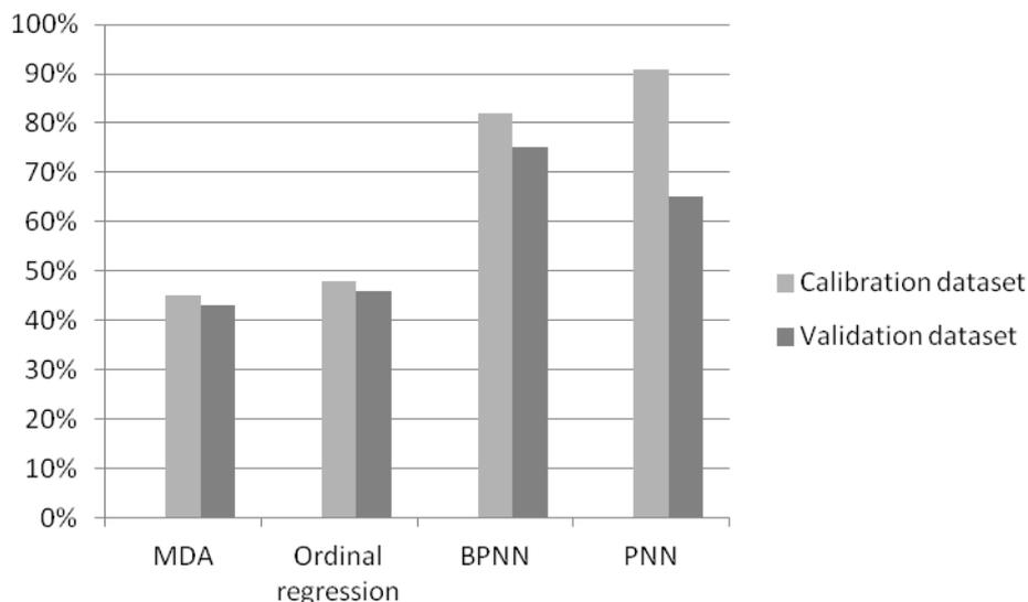
Figure 11: Total model efficiency  $E_{tot}$  for the application of the pipe level models in the City of Greater Dandenong (adapted from Tran (2007))
