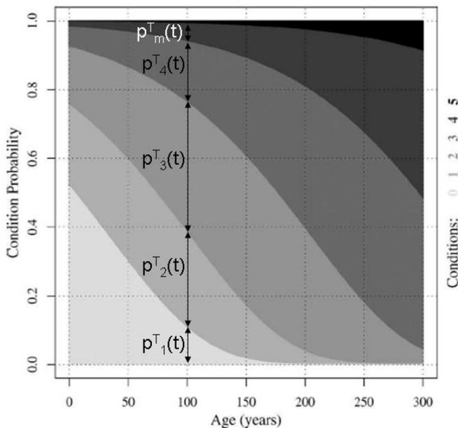
Figure 6: Gompertz condition survival functions related to a stormwater concrete pipe of the Dresden sewer system, Germany, and an example of a state vector at age 100 (from Le Gat (2008))
