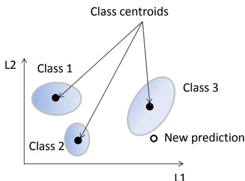
Figure 7: Illustration of a discriminant analysis classification with three condition classes (adapted from Tran (2007)).
