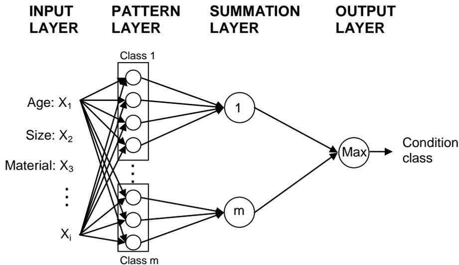
Figure 9: Schematic presentation of the probabilistic neural network PNN (adapted from Ana (2009))
