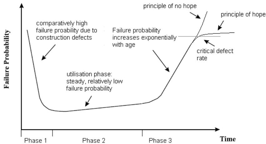
Figure 4: ‘Bath tube’ curve (from Herz, 1999): graphical description of the deterioration process
