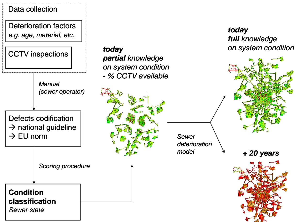
Figure 1: From CCTV inspection programs to sewer deterioration modeling. The condition evaluation of the available CCTV reports gives only a partial knowledge about the system condition. These condition data are used as input data to calibrate deterioration models and perform new predictions.
