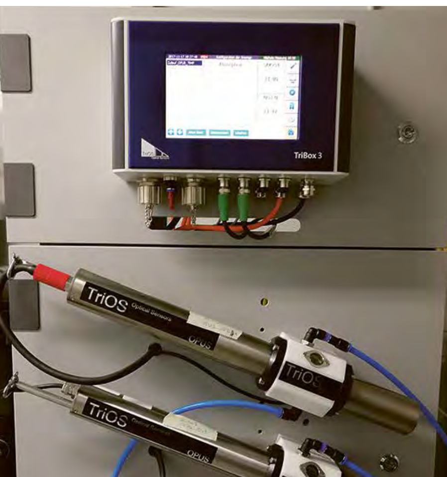
UV-VIS-Sensors installed in the ozone pilot plant
