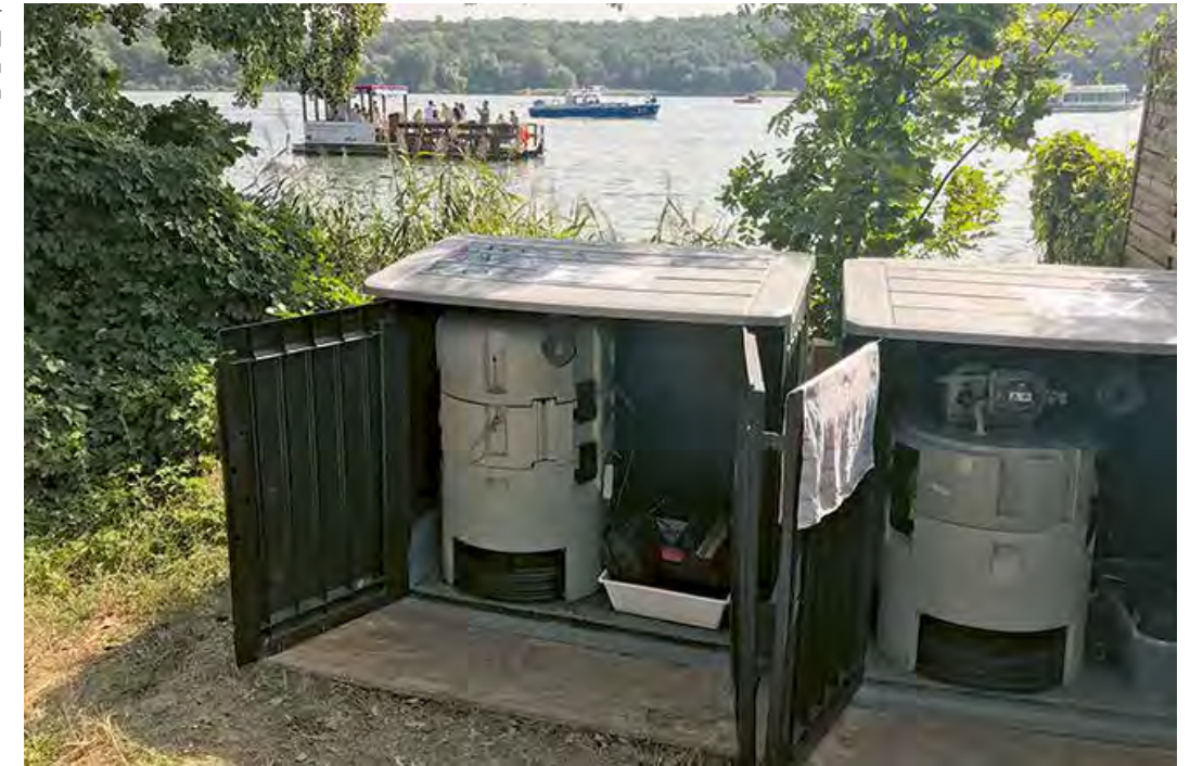
Automatic sampler for microbiological control of the forecast model on River Havel in Berlin
