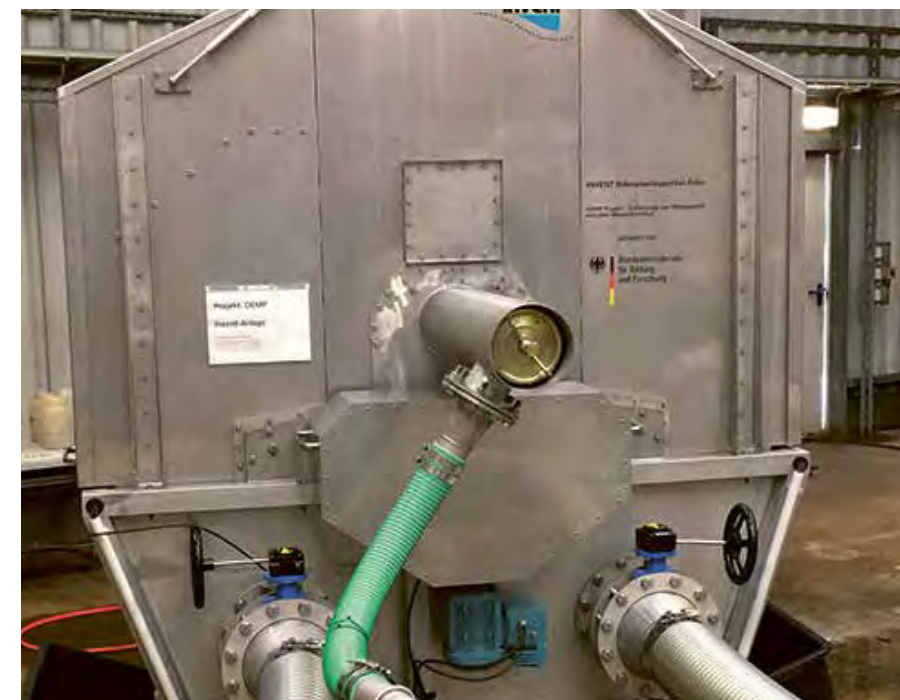
Pile cloth media filtration pilot unit at WWTP Berlin-Ruhleben
