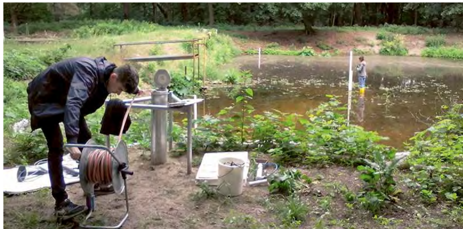
Measurement of temperature profiles in a groundwater infiltration plant
