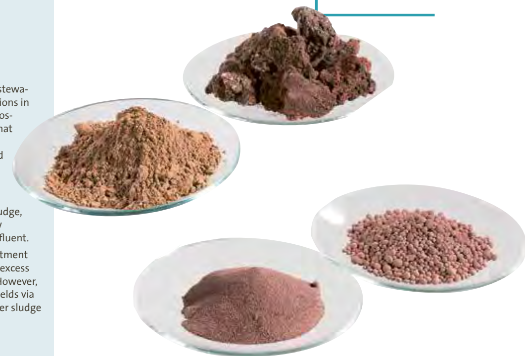
Intermediate substances during manufacturing of granulated Phosphorous recycling products from sewage sludge ash
