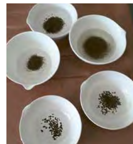
Results of laboratory and pilot tests with granulated sewage sludge (b.l.)
