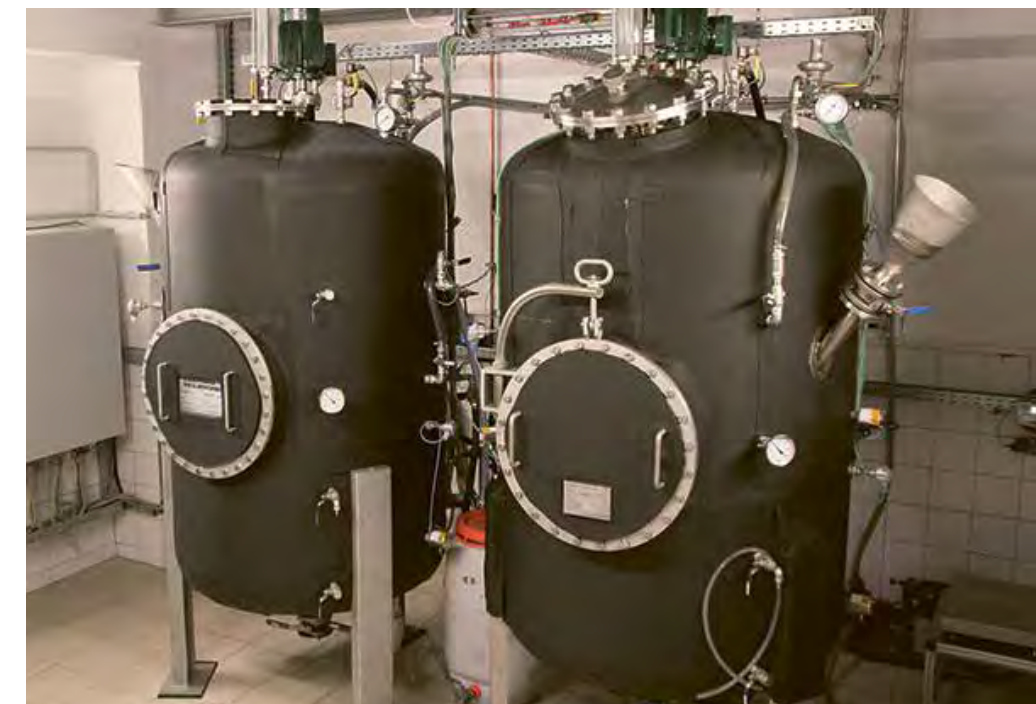
Pilot reactors for thermo-pressure hydrolysis with sewage sludge (right)
