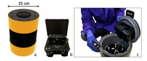
Figure 1: In situ ALERT System; b – ALERT Lab portable/bench-top instrument; c – View of the ALERT System during field maintenance operations (adapted from [Angelescu et al 2020b])
