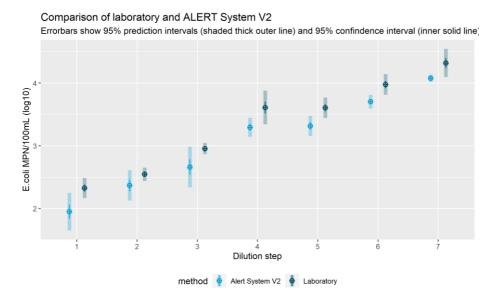
Figure 56: Repeatability study results. The plots show prediction (outer, thick, shaded interval) and confidence interval (inner, solid) of the ALERT System V2 and the laboratory.
