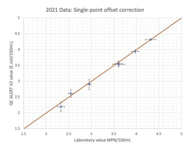
Figure 59: The side-by-side data for ALERT V2 from the 2021 repeatability study, after applying a single-point offset removal by subtracting the offset measured at the highest concentration (where ALERT V2 shows the best precision). The error bars represent the standard deviation. 95% confidence intervals correspond to 1.96 x standard deviation.
