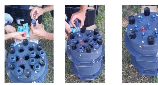
Figure 36: Set up of the cartridges in ALERT V2
