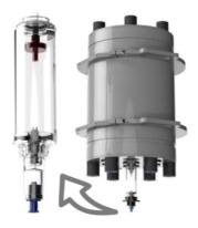
Figure 3: The ALERT V2 instrument, including a zoom on the sampling cartridge, at left. The cartridges are inserted in the instrument from the bottom, theirs sampling check valves being immersed in the water body of interest. Regarding the cartridge, from top to bottom we can identify the vacuum sampling port and hydrophobic filter, the transparent reaction chamber, the diffuser and isolation check valve, the reagent chamber and the sampling check valve.
