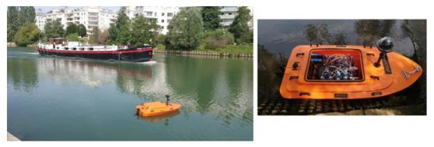
Figure 18: Fluidion DRONE usage for sample collection for performing spatial variability analysis in Marne river
