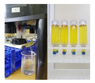
Figure 30: Left side: Sampling with cartridge 1 using a barb adapter with a tube. In the background: external temperature sensor. Right side: Filled sample cartridges after analysis.
