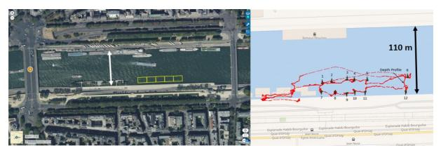
Figure 20: Fluidion DRONE recorded GPS trace and sampling locations in the Seine River
