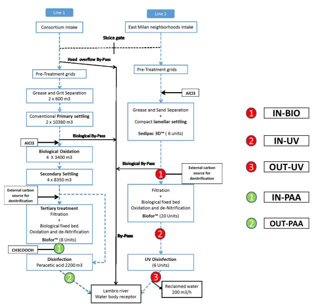
Figure 32: Peschiera Borromeo WWTP and sampling points for ALERT Lab testing
