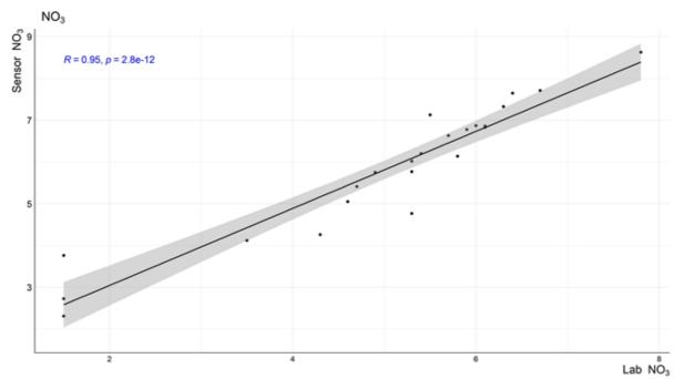
Figure 31: Correlation between nitrate measurements obtained by sensor and laboratory analyses in Pero WWTP
