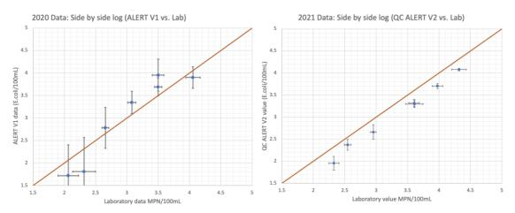
Figure 58: Comparison of the 2020 Alert V1 vs. Lab repeatability data (left figure) and 2021 Alert V2 vs. Lab repeatability data. The improvement in both linearity and precisions for the ALERT V2 is immediately visible. Also visible is the quasi-constant small bias observed in 2021 over the full concentration range. The error bars represent the standard deviation. 95% confidence intervals correspond to 1.96 x standard deviation.
