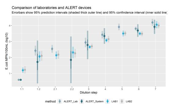
Figure 53: Replication study results. The plots show the individual measurements of the two accredited laboratories (LAB1, LAB2) (N = 12) and the two ALERT devices (ALERT\_Lab, ALERT\_System) (N=6, N = 7)
