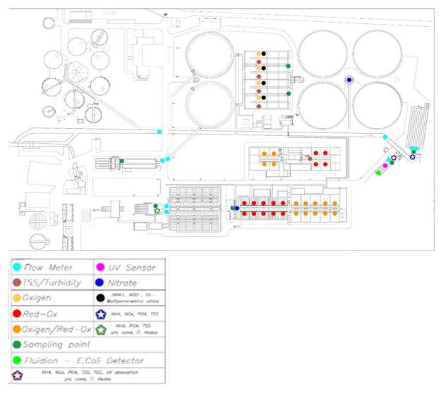
Figure 7: Sensors installed at Peschiera Borromeo WWTP
