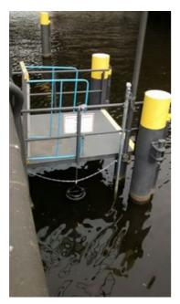
Figure 28: Fluidion ALERT System V1 installed in Spree-Canal for DWC campaign in 2019
