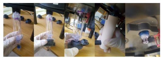
Figure 29: Maintenance of the ALERT System V2; Replacement of the sample cartridges.
