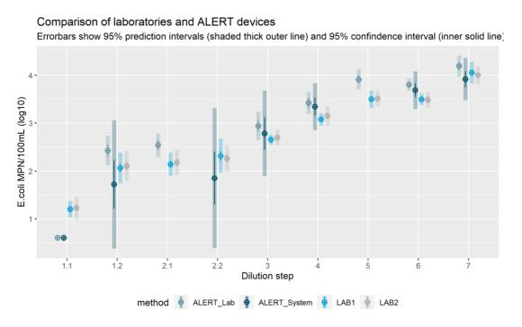
Figure 55 - Repeatability study results. The plots show prediction (outer, thick, shaded interval) and confidence interval (inner, solid) of the two ALERT devices and the two laboratories.
