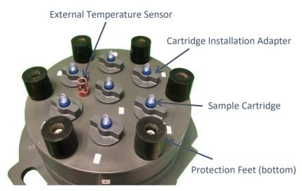
*Figure 6: Upside-down view of the instrument's bottom interface, showing the protection feet, the seven cartridge sampling ports, and the external temperature sensor.*
