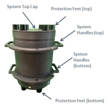
*Figure 5: The external mechanical details of the ALERT V2 instrument. The sampling ports are located at the bottom of the instrument.*
