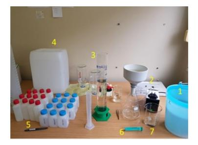
*Figure 27: Material used for conducting the replication. 1: Sample of secondary effluent, 2: filtering equipment, 3: measuring cylinders, 4: 20 L canister, 5: PE bottles for the two laboratories, 6: Syringe, 7: beaker*
