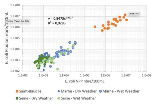
Figure 41: Comparison between ALERT and laboratory data for all combined deployments in Paris area (including surface water during dry and wet weather, as well as stormwater outflow monitoring)
