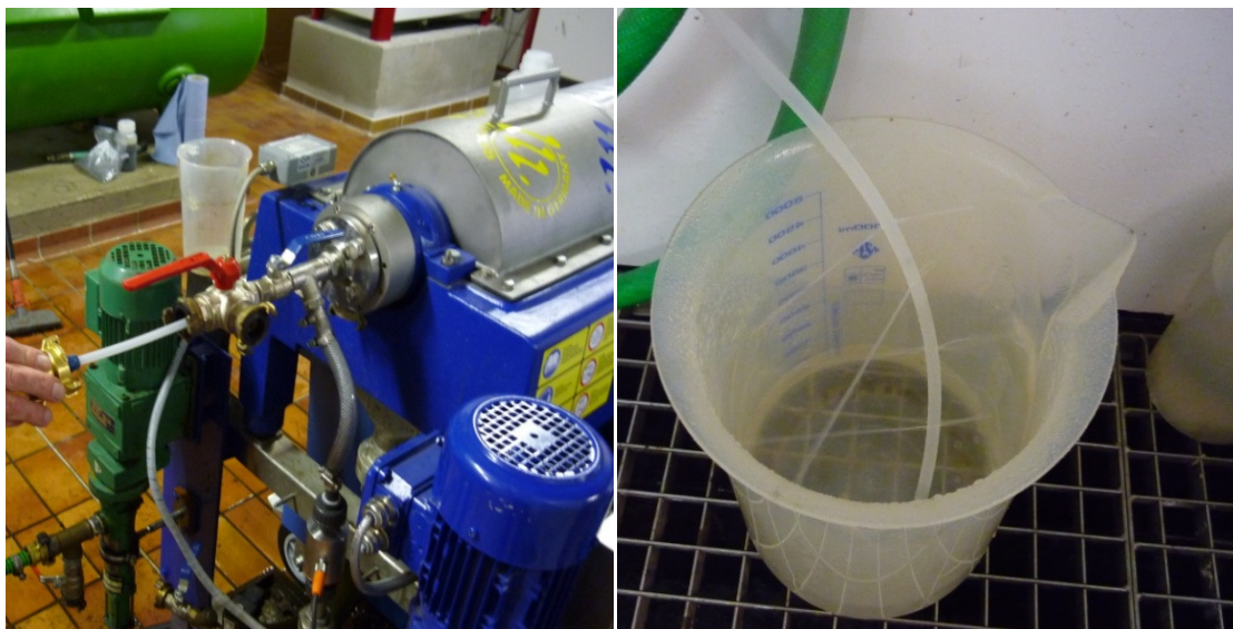
Figure 4-1: Insertion of the polymer feeding tube in the screw (left) and close-up of polymer solution spraying out of the perforated tube (right)
