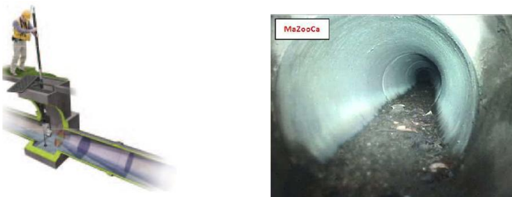
Figure 5: left: QuickView® System ; right: an example of visual screening done with a zoom camera (Ertl, 2012)
