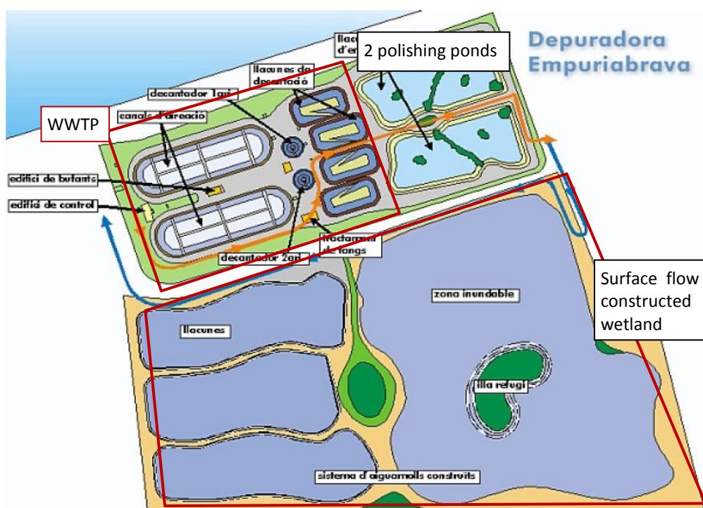
Figure 19: Empuriabrava WWTP with subsequent polishing ponds and surface flow constructed wetland (from Pallarès 2009)
