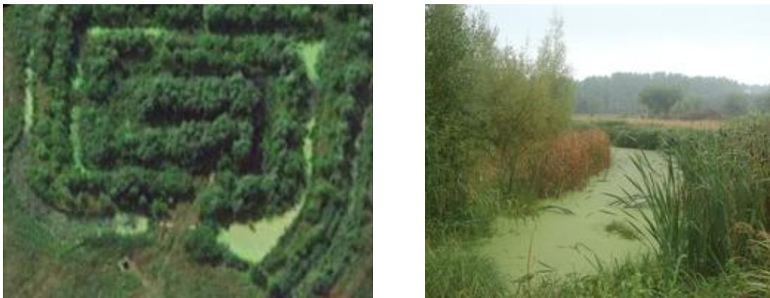
Figure 13: Spiral-shaped FWS wetland in Berlin-Hobrechtsfelde – left: top view (source: Google Maps), right: outer part of spirale wetland (photo taken by author).
