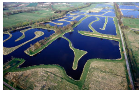
Figure 5: Meander system of infiltration fields
