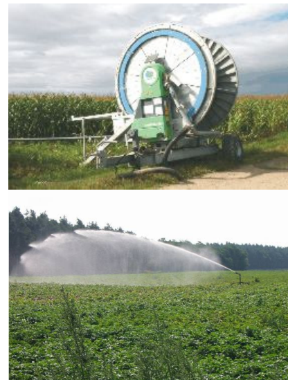
Figure 6: Irrigation machinery for spreading of reused effluent
