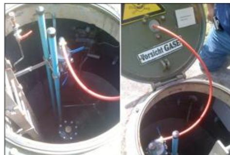
Fig.14: Modified robbins device
