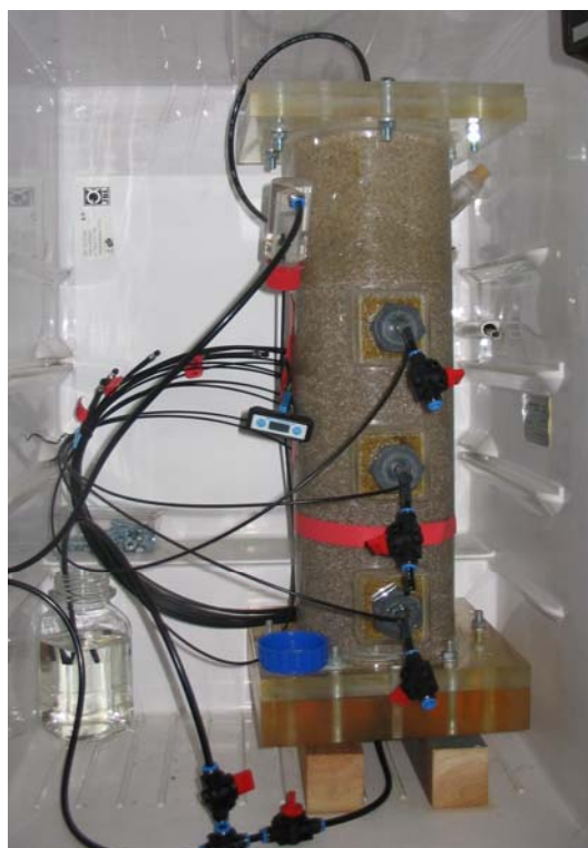
Figure 117 Picture of the set-up used for the investigations of temperature influence
