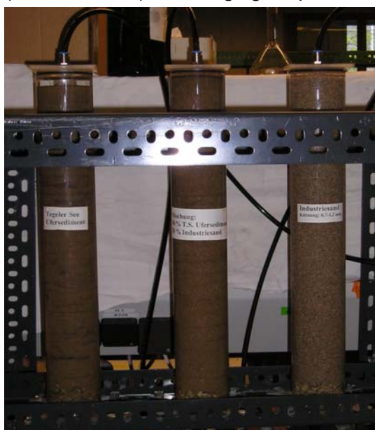
Figure 138 Soil columns for the determination of the retardation factor
