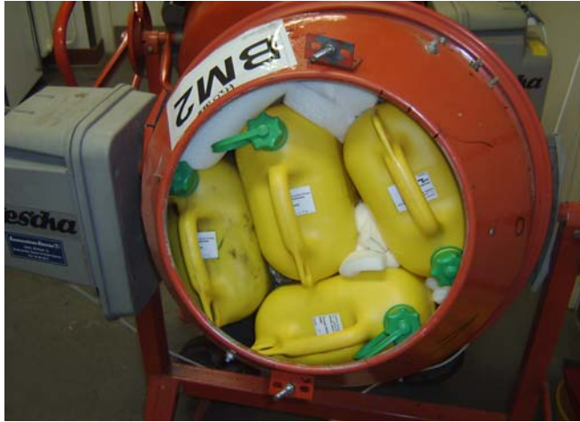
Figure 114: Concrete mixer with firmly packed petrol containers. For agitating it was additionally covered.
