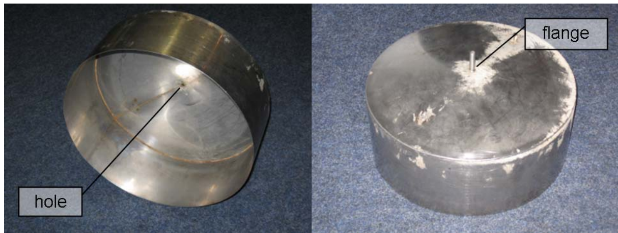
Figure 1 Barrel used for direct infiltration measurements. The open bottom is pushed into the ground, a hose with the reservoir bag is plugged to the flange at the top.
