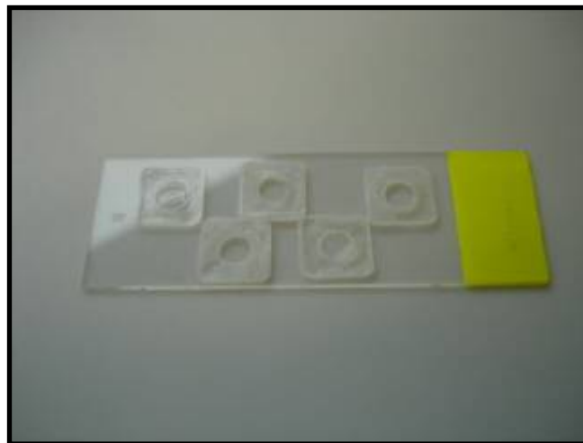
Figure 28: glass slide with a two week old biofilm with grommets used as hybridization chambers
