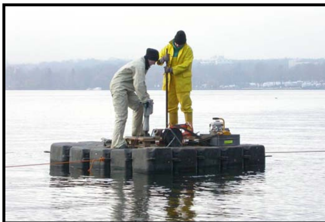
Figure 50: Taking cores from the drilling platform at Lake Wannsee.
