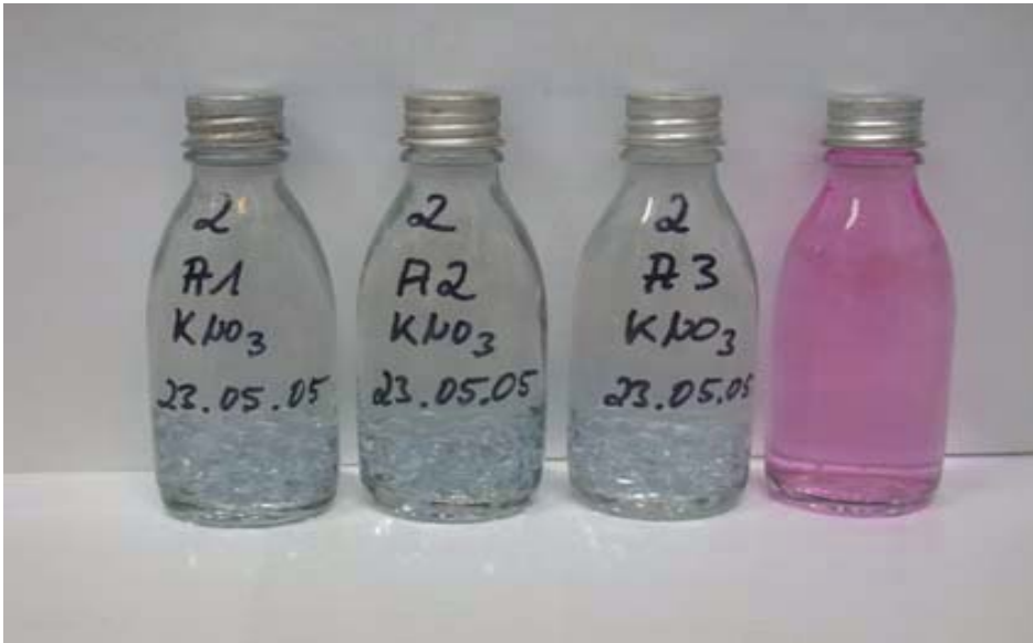
Figure 12: Screw cap tubes filled with sulfide reduced anoxic medium supplemented with KNO 3 . The pink bottle shows an example of oxidized medium.
