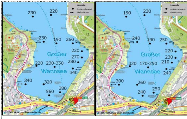
Figure 77. Primidone concentrations [ng/L] across lake Wannsee in March (left) and July (right) 2004
