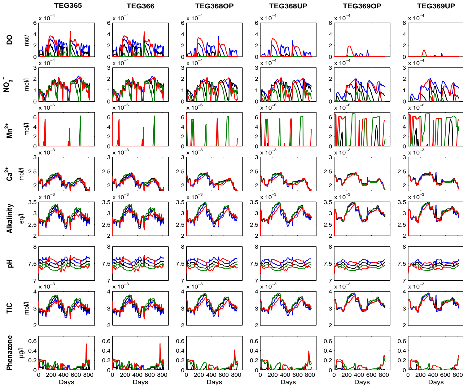
Figure 67 Temperature dependence of dissolved oxygen (DO), nitrate, \text{Mn}^{2+} , calcium, alkalinity, pH, TIC and phenazone at the monitoring wells TEG365, TEG366, TEG 368OP/UP and TEG396OP/UP. The blue, black and green lines represent simulations with constant temperatures of 5°C, 10°C and 15°C, respectively. The red lines represent the final calibrated reactive transport simulation (variable temperature).
