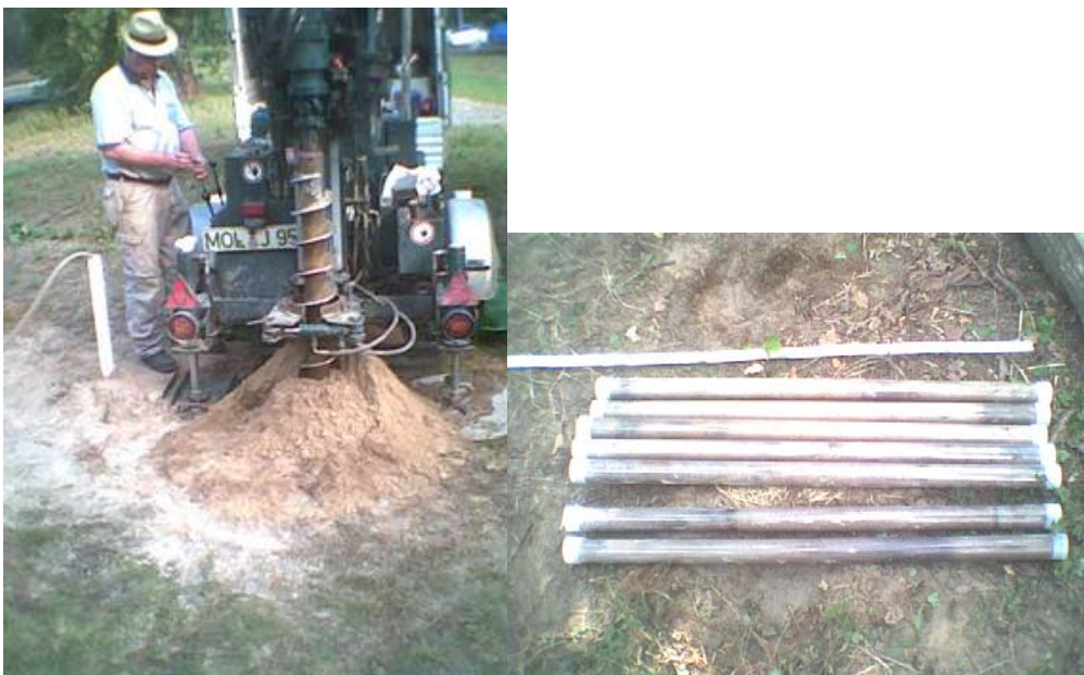
Figure 1: Snap shot of NORDMEYER drill (left) and recovered plastic liner containing aquifer sediment (right).
