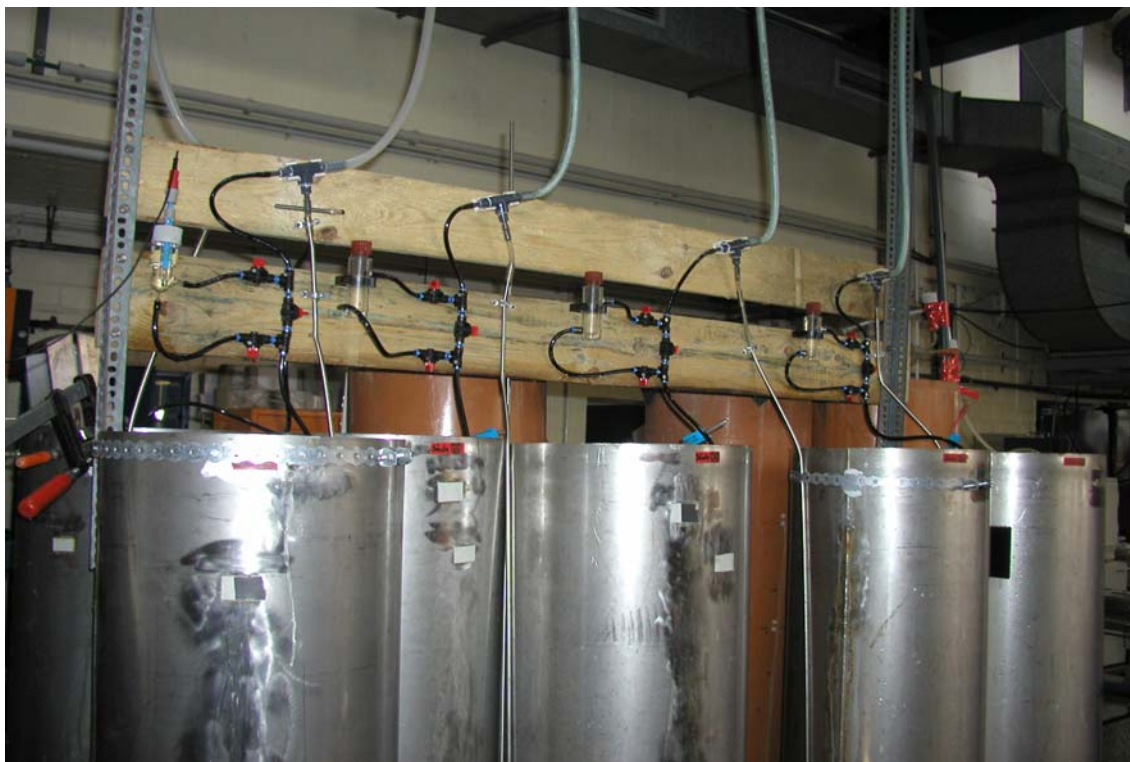
Figure 70 Long retention soil columns Marienfelde (top part)
