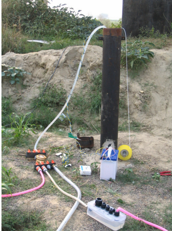
Photo 5 Measuring setup at a piezometer (flow-through cell, accumulator, light plummet, water meter)
