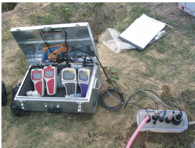
Photo 6 Measuring in-situ parameters on site (flow-through cell, measuring devices in steel box).
