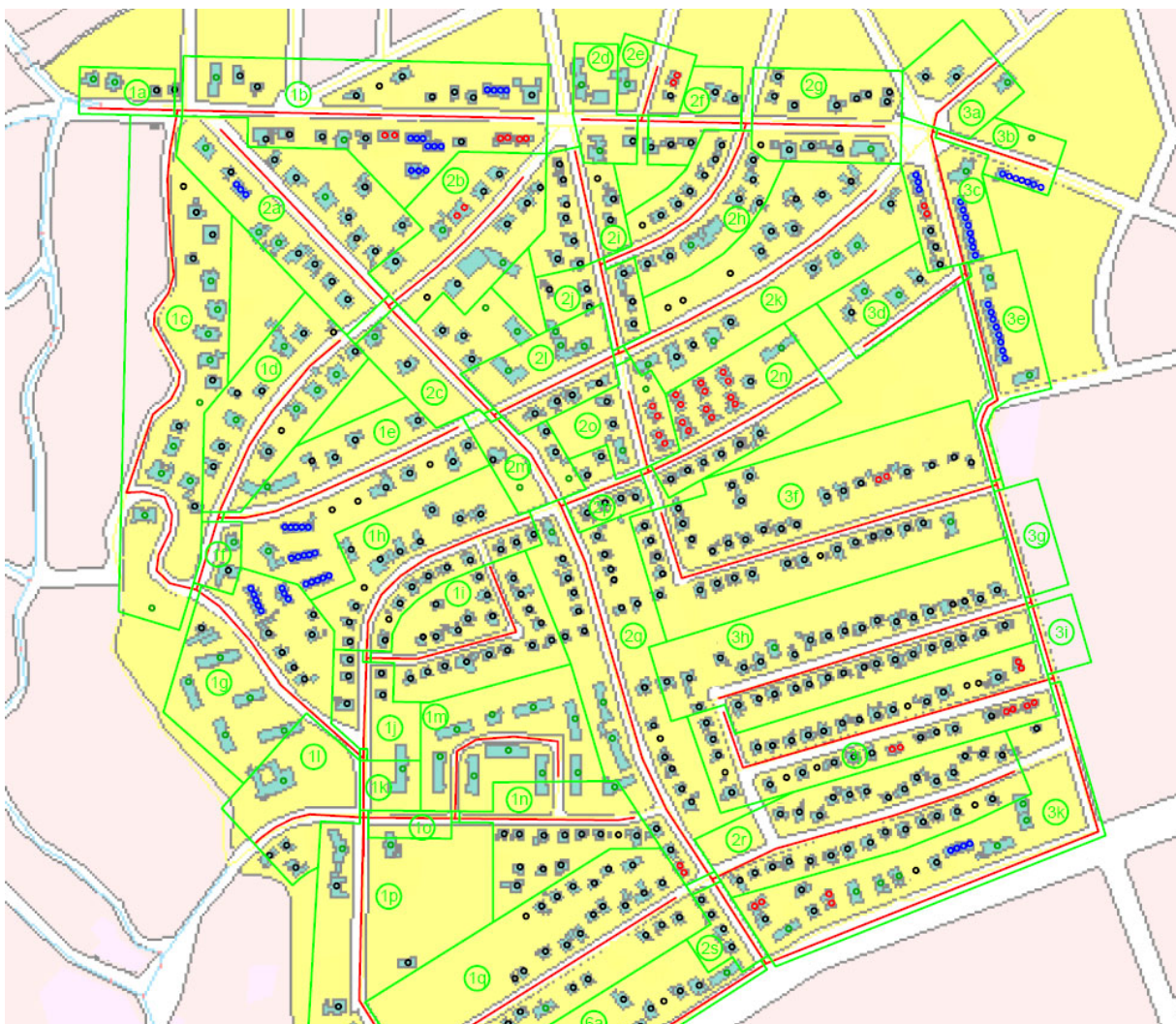
Figure 61: Exemplary layout of the conventional sewer system in the northern part of the study area (Red: sewage pipes, green: sections of drainage area)
