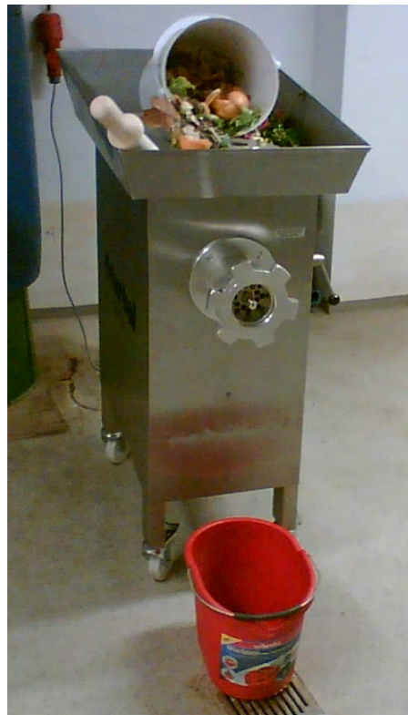
Fig. 2.4.22: Grinder (Edertal 2007) for bio-waste for biogas plant
