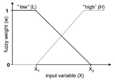
Figure 5 Fuzzy classification of input parameters (taken from Schärer et al., 2006)
