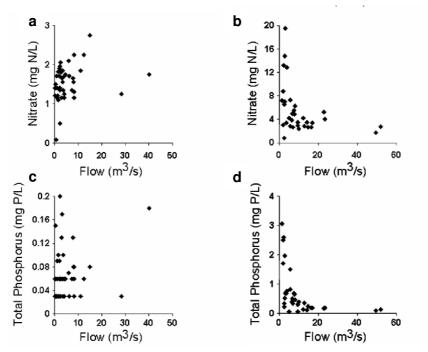
**Figure 1** Relationship between flow (Q) and water quality parameters ( $NO_3$  and total P) from Albek (2003); (a) and (c) showing the concentrations at the rural monitoring station; (b) and (d) showing the concentrations at the urban station.
