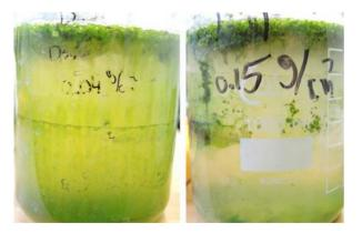
Figure 20: Comparison of algae formation at different mat densities from 03.03.-09.03.2017: Left beaker: Mat density 0.05 g·cm<sup>-2</sup>; Right beaker: Mat density 0.15 g·cm<sup>-2</sup>
