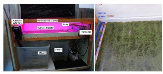
Figure 8 Left: Laboratory pilot plant; Right: duckweed reactor including barrier and harvest groove (blue and red coloured)
