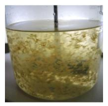
Figure 11: Filtrate after flocculation and precipitation prior to sieving (100µm)
