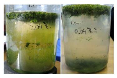
Figure 23: Formation of submerged algae in beaker with duckweed mat density of 0.05 g⋅m<sup>-2</sup> without side cover (left picture; 16.02.2017) and with side cover (right picture; 10.03.2017)
