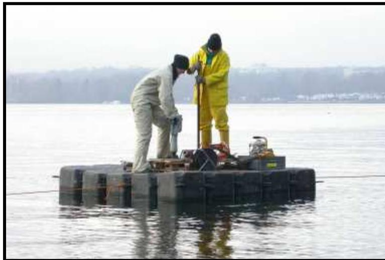
**Figure 55: Taking cores from the drilling platform at Lake Wannsee.**
